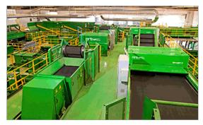
GreenWaste Recovery has opened a new materials recovery facility (MRF) at its San Jose, California, location. The MRF was designed, manufactured and installed by Eugene, Oregon-based Bulk Handling Systems (BHS) to process commercial and residential single-stream recyclables at rates in excess of 40 tons per hour (tph).
