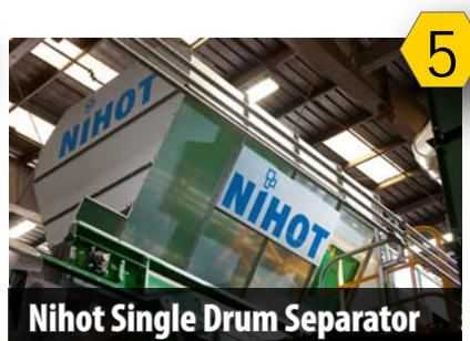
Nihot Single Drum Separator Separates glass from fiber fines
