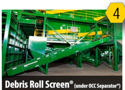
Debris Roll Screen® (under OCC Separator®) Breaks glass and separates fines (including glass) from paper and containers
