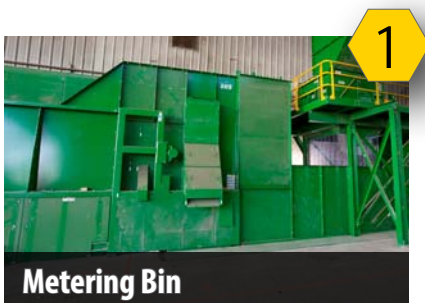
Metering Bin Provides an even, steady flow of material into the system.
